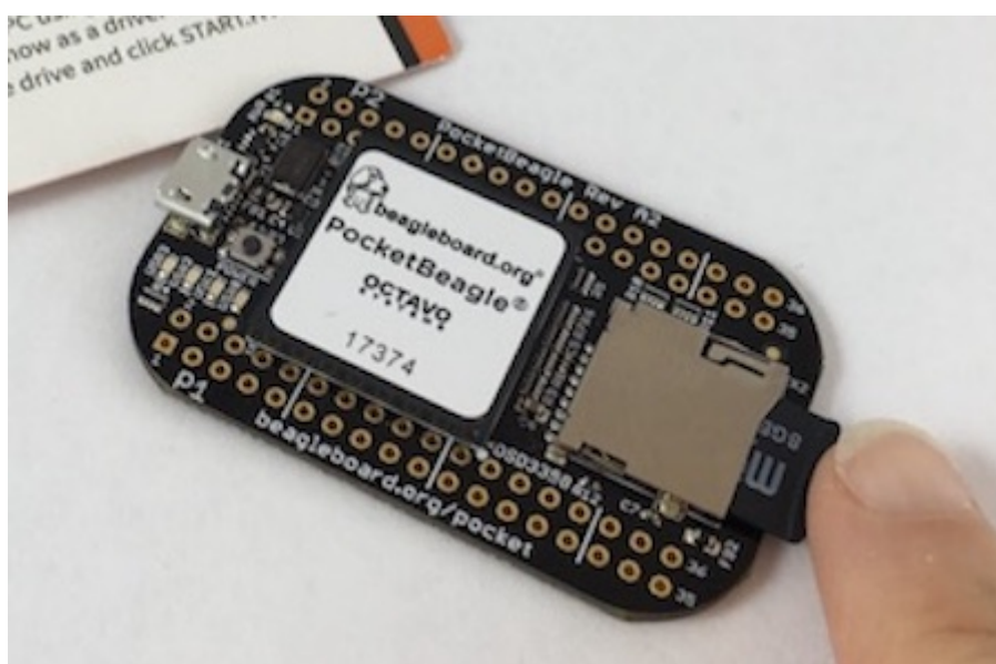
Fig. 2.11: Insert the microSD Card into PocketBeagle
