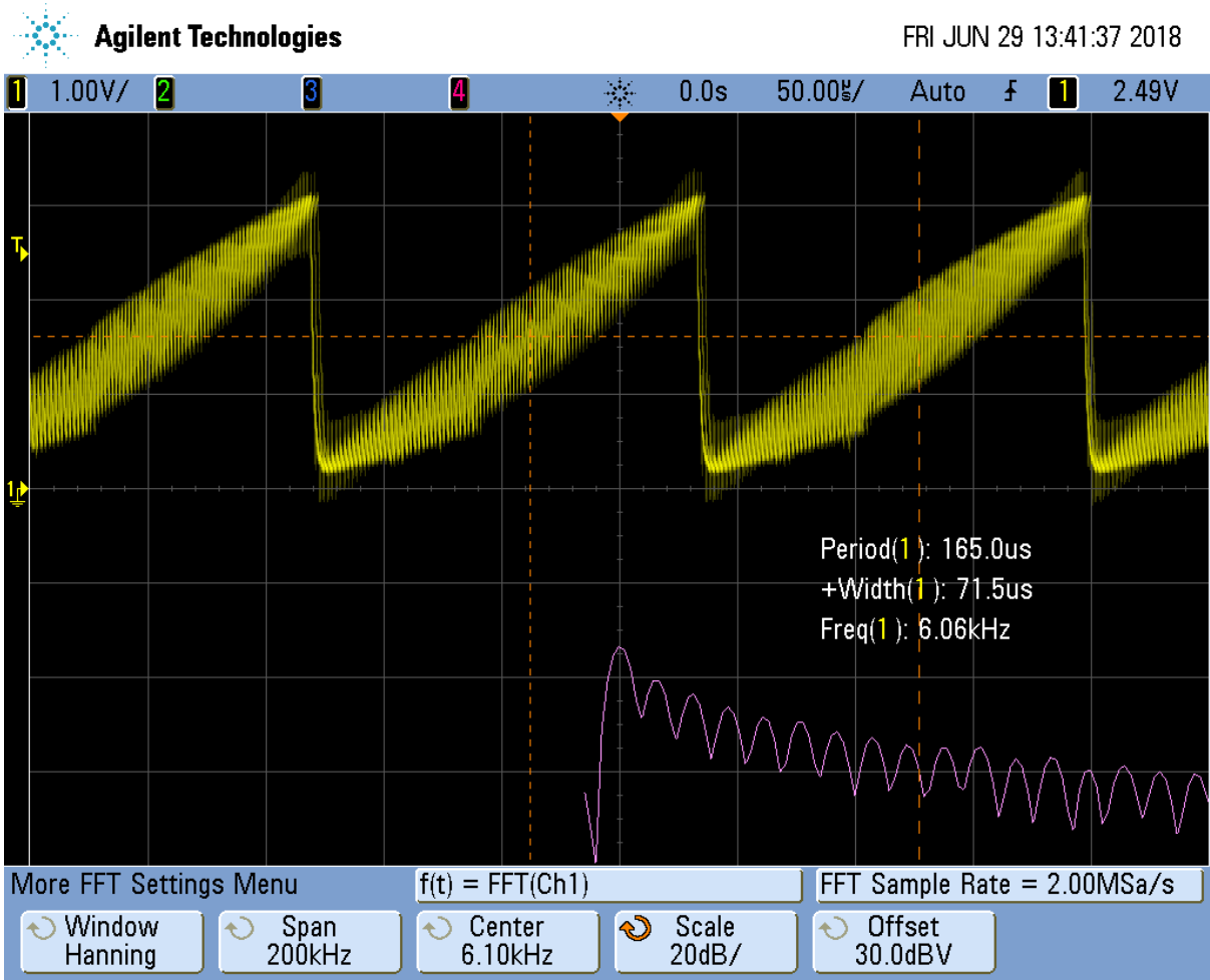
Fig. 4.166: Reconstructed Sawtooth Waveform with Higher Cutoff Frequency
